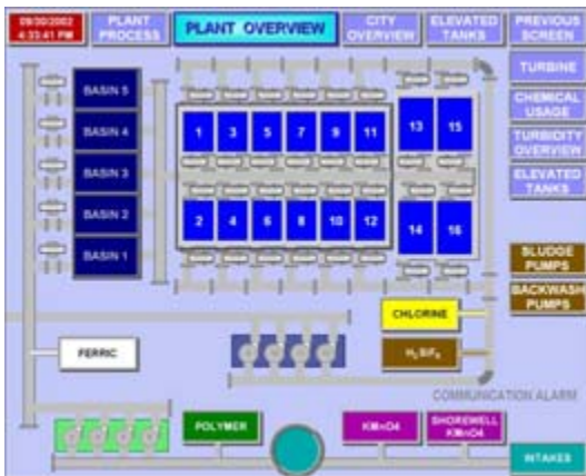
Plant Overview Screen
